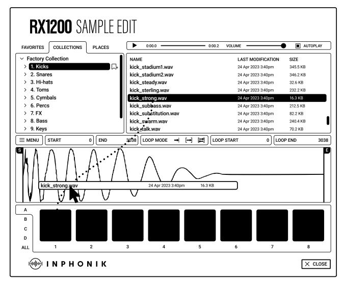
Click the red "Sample" button to access the Sample editor. This interface displays a file browser, a sample editor and the RX1200 pads for assigning samples with drag-and-drop gestures.
